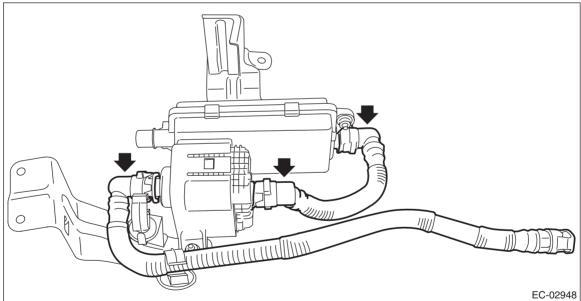
3) Install the drain separator to the leak check valve assembly. <Ref. to EC(H4DO(w/o HEV))-62, INSTALLATION, Drain Separator.>
