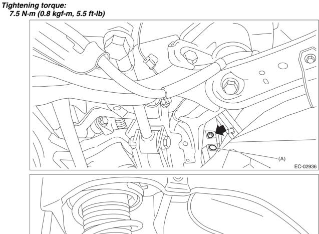
2) Connect the connector to the leak check valve assembly.
