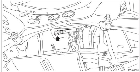
10) Disconnect the fuel filler hose (A) and evaporation hose (B).
