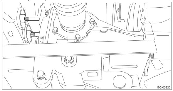
7) Temporarily tighten the self-locking nuts which hold the rear differential to the rear sub frame assembly. NOTE:
