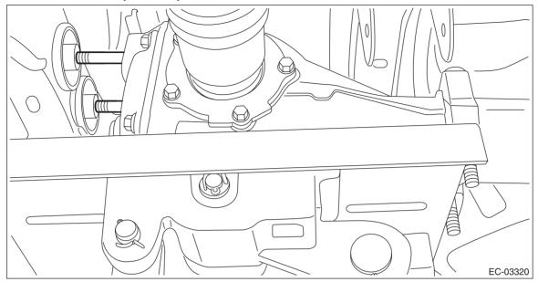
• Do not lower the rear differential excessively. Doing so may add extra load to the drive shaft or cause the falling-off of the drive shaft.
