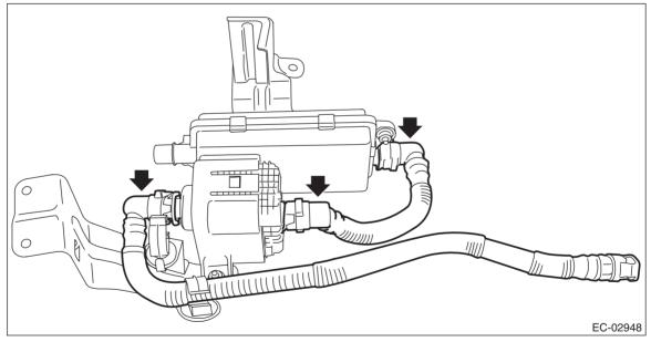
3) Remove the bracket from the leak check valve assembly.
