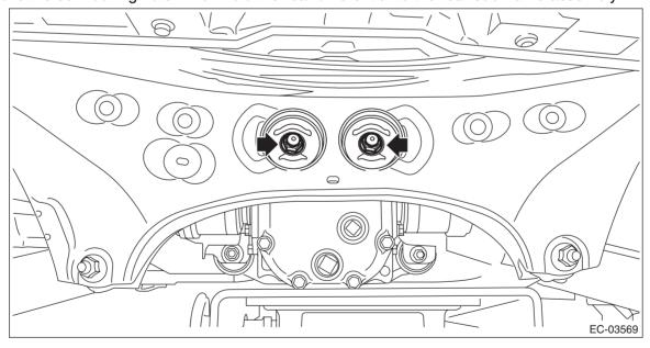
7) Remove the rear differential member from the rear sub frame assembly and the rear differential.
