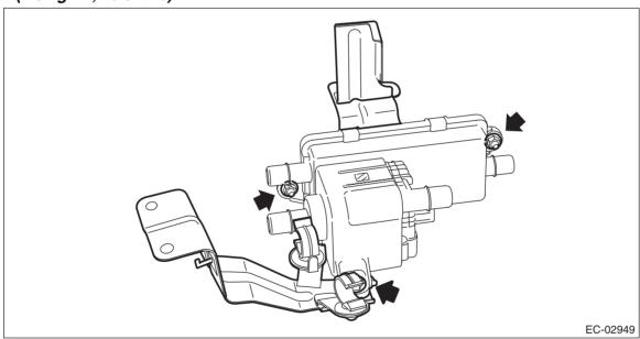
2) Install the drain tube to the leak check valve assembly.
