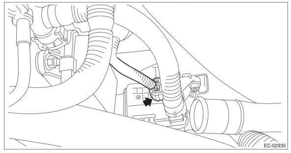
13) Remove the bolt and clip (A) which secure the leak check valve assembly to the vehicle, and remove the leak check valve assembly.
