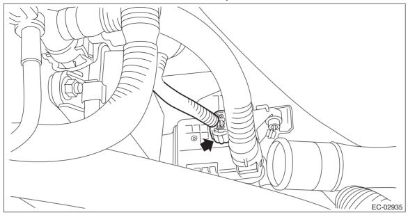
3) Connect the intake hose (C) to the connector.
