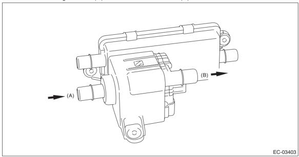
3) Connect the battery positive terminal to the terminal No. 5 and the battery negative terminal to the terminal No. 1. Check that air does not come out from (B) when air is blown into (A).
