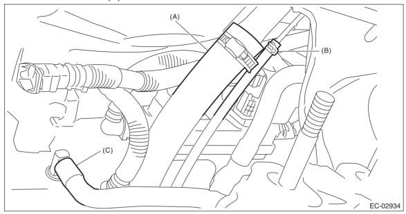
12) Disconnect the connector from the leak check valve assembly.
