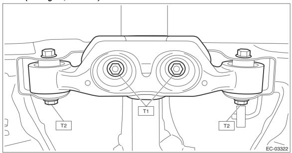
11) Tighten the self-locking nuts which secure the rear differential to the rear sub frame assembly.
